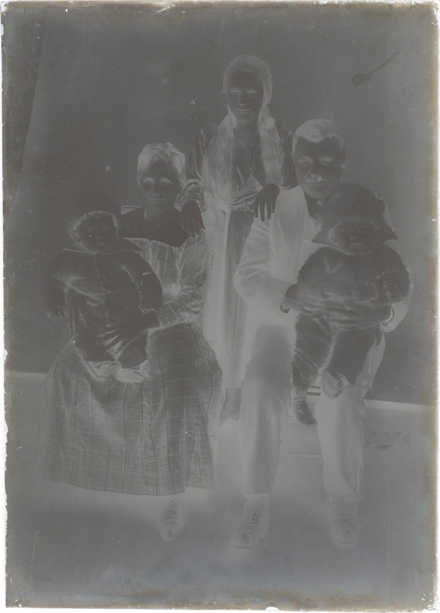
Image 2.15: A gelatin glass negative. Note the blue cast of silver mirroring on the bottom and right edges.
